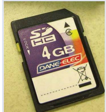
An SD (Secure Digital) memory card is a storage medium for digital photos. Digital cameras are often packaged with low-capacity SD cards; many people buy larger SD cards so they can use their camera longer without filling the card up or they carry multiple SD cards with them on extended trips. The card is easily removed from the camera.
